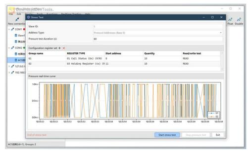
is an all-in-one tool designed to manage and debug Modbus communications across multiple devices and protocols. It supports various Modbus protocols, including RTU, ASCII, and TCP/IP, allowing you to create multiple connections at once and monitor data from various slave devices. The tool is particularly useful for testing function codes and ensuring your Modbus systems are set up correctly without needing to edit raw data frames manually.
