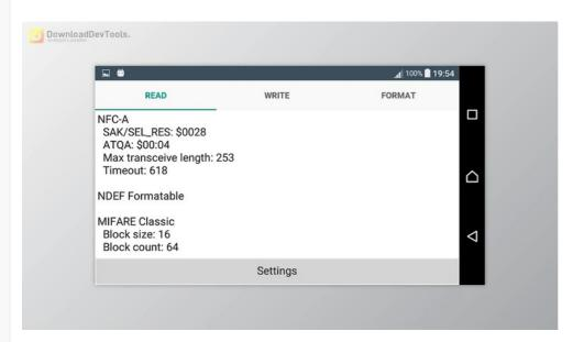
Winsoft NFC Library for Android is a comprehensive solution designed specifically for Delphi and C++ Builder developers seeking to incorporate NFC functionality into their Android applications. Leveraging the Android NFC API, this library facilitates seamless reading, writing, and formatting of NFC tags, providing robust support for various tag types, including ISO-DEP, NDEF, NFC-B, NFC-F, NFC-V, MIFARE Classic, and MIFARE Ultralight.
