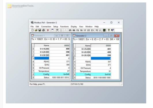
Modbus Poll is a specialized simulator for Modbus master developers and those testing the Modbus protocol. A multiple document interface enables simultaneous monitoring of various Modbus slaves, supporting different protocol variants like RTU, ASCII, TCP/IP, and more. The tool simplifies parameter specification for monitoring, making it versatile for industrial applications
